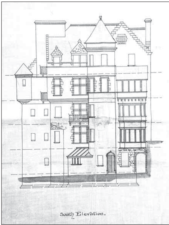
Fig. 5. South elevation of the 'double tenement' in the south west corner, Ramsay Garden: Comparison with the 2013 photograph (fig. 4) showed a host of minor variations. (ECA, Dean of Guild Plans , 11 June 1892.)
