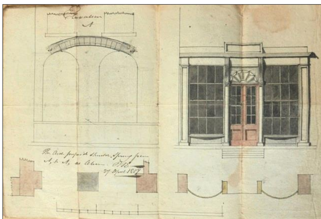
Description: a. Before and after elevations and plan of the front wall. Size: 22.0 x 33.4 cms. Inscriptions, recto: (Signed) RB(?) 27 April 1807. Architect: Robert Burn?
