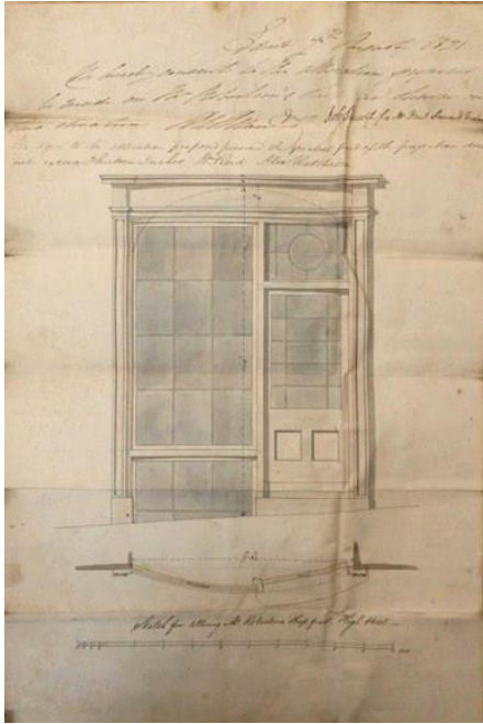
Description: a. Elevation and plan of the shop front. Size: 21.0 x 29.3 cms.
