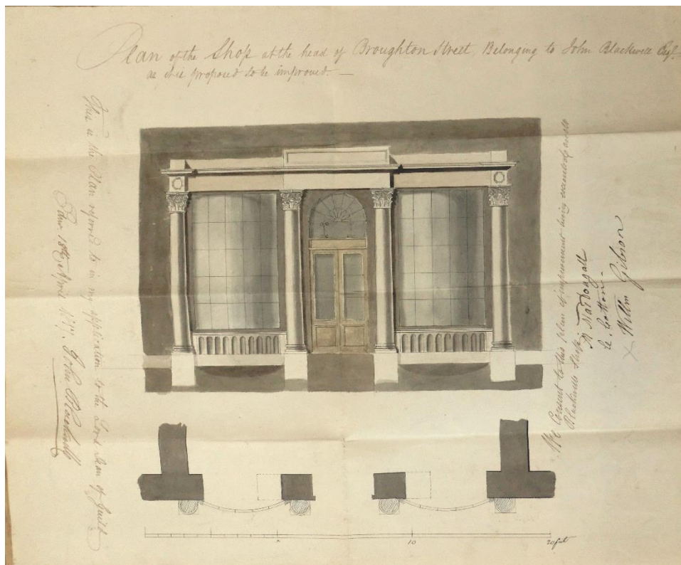
Description: a. Elevation and plan of the shop front. Size: 28.2 x 34.5 cms.
