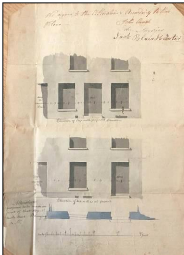
Description: a. Elevations of the shop floor, before and after with a plan of the front wall. Size: 34.3 x 24.0 cms.
